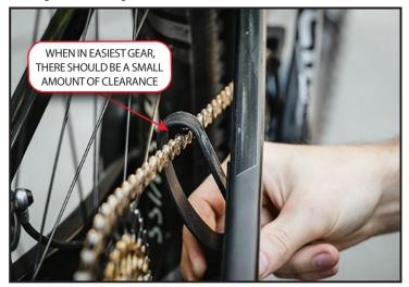
8. If the chain is rubbing in the hardest gear and sliding the STFU towards the cranks (10 mm or so) doesn't fix this then trimming the height of the STFU by 5mm may be required. Before doing so, make sure there is sufficient room between the chain and the top of the STFU when in the easiest gear (biggest cog) - you may need to move the location of the STFU closer to the cranks to accommodate this.
