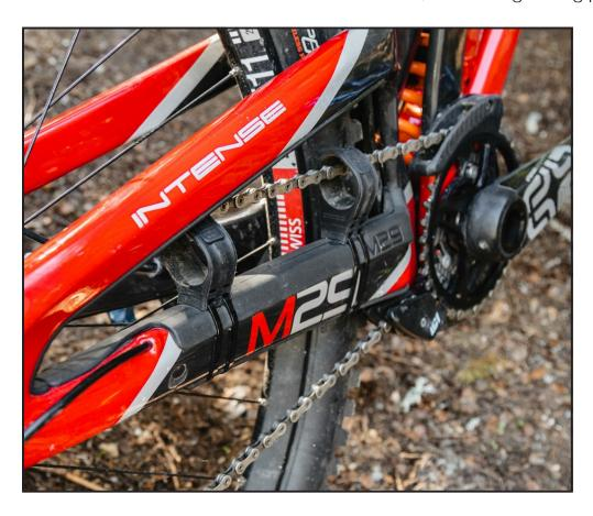
**▼ Gearing:** The STFU chain dampers are designed to work with 1 X setups only. This means if you have more than one front chain ring the system will not function as designed. We have tested using a single larger unit of the TRAIL set with 2X setups (2 front chain rings) and it works on some bikes. We recommend our STAY-GUARD protection tape for 2X and 3X setups.
